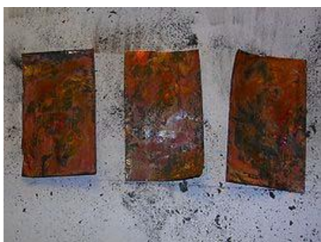
Figure (1) (c)- scraped black cupric oxide revealing cuprous oxide underneath.
