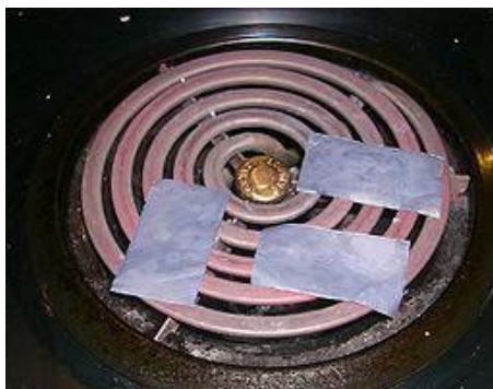
Figure (1) (b)- copper coated with cupric oxide.
