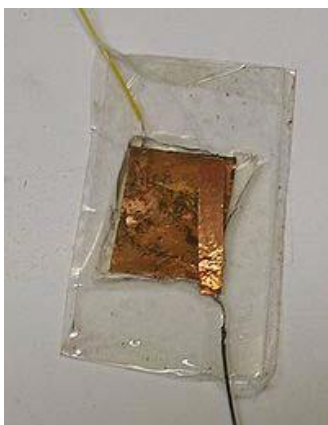
Figure (3) The package of cuprous oxide solar cell.
